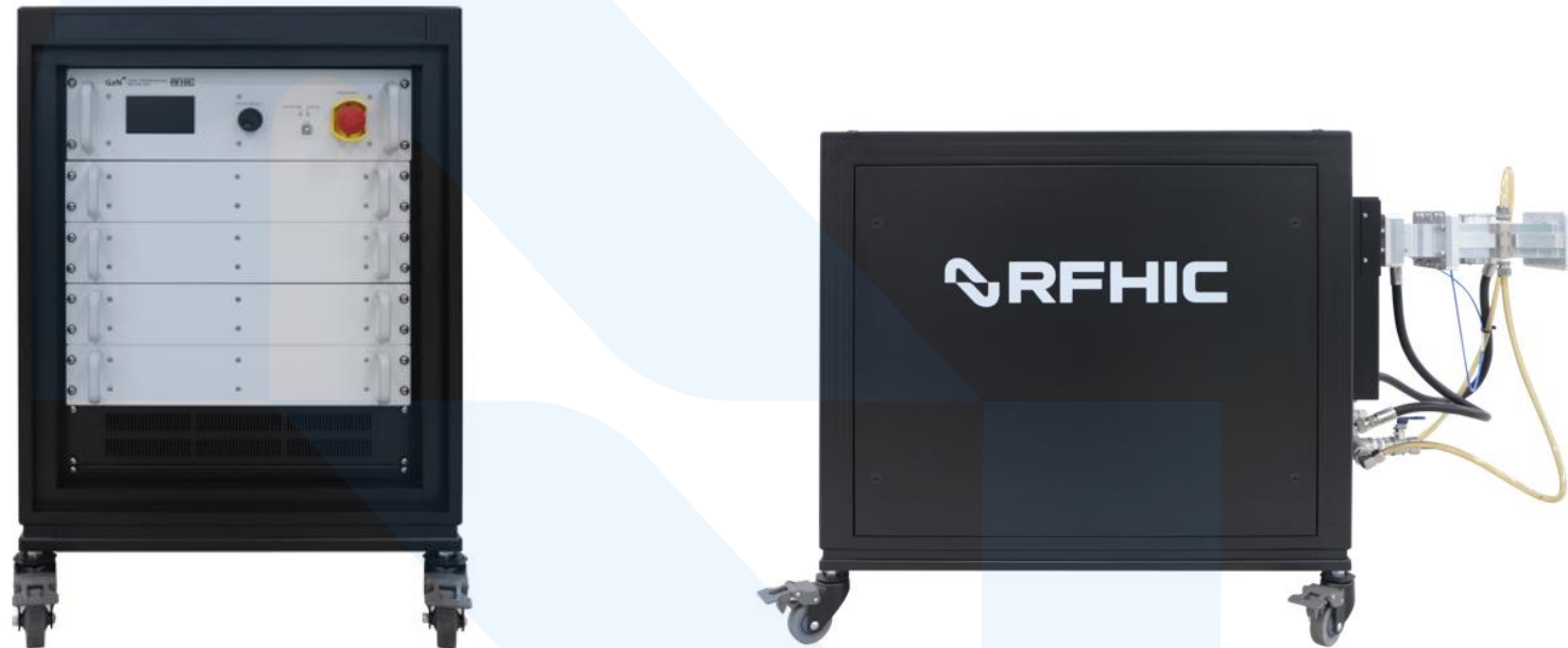
Figure 1: RIK2512K-40TG_H GaN SSPA Head Front & Side View
